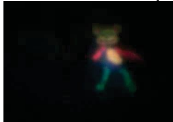
Fig. 4. 3D color bear reconstructed from transmitted hologram data.
