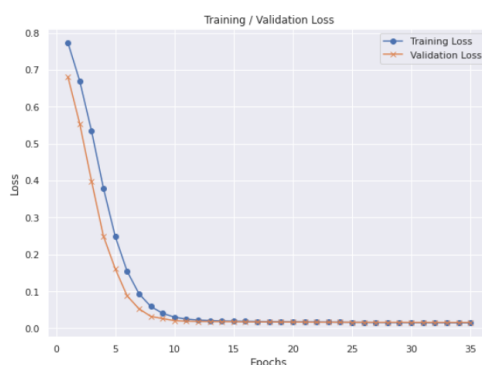
Fig 1: Training and validation losses of the model with 1 hidden layer over the epochs
