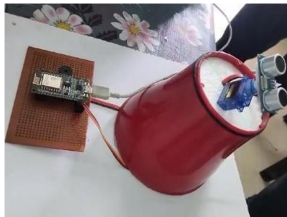
Fig.3.The smart sensor setup mounted on Servo motor.
