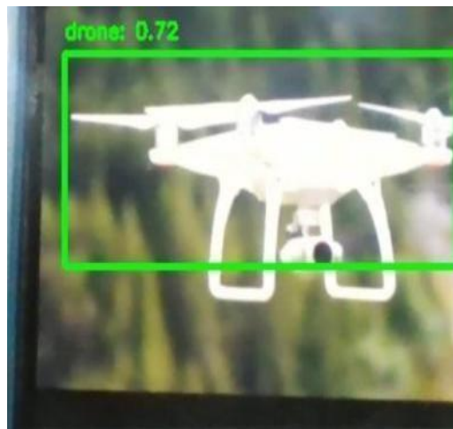
Fig.4. Drone Detection in action: A detected drone with 72% confidence.
