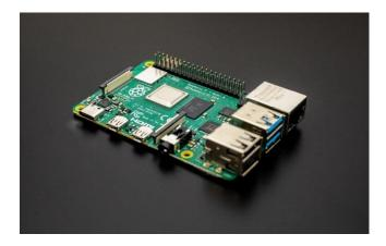
The Raspberry Pi 3B+ is the main component of our project, selected for its compact size and high performance. This device serves as the central hub for controlling the SDS011 sensor and processing the incoming data. The Raspberry Pi runs on the Raspberrian operating system, which is optimized for its hardware and provides a reliable foundation for our python 3.8 scripts. Together, these elements provide a powerful and flexible platform for our project.
