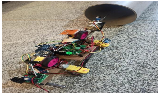
Fig 3.1: Proposed Pipeline Inspection Robot
