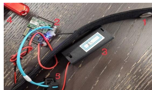
Fig. 9 TGAM brainwave headband and Bluetooth adapter; sensor (1), TGAM chip (2), bluetooth module (3), battery box (4), and bluetooth adapter (5).
