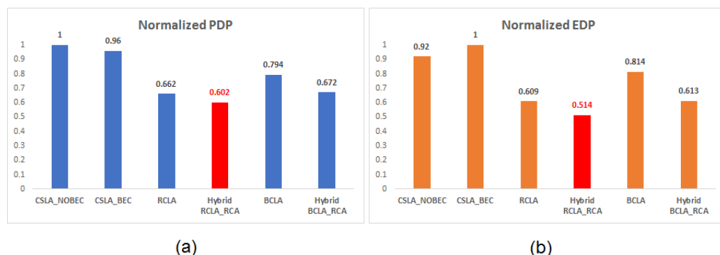
Figure 4. Normalized (a) power–delay product (PDP) plots, and (b) energy–delay product
