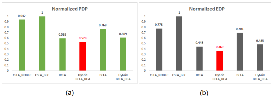
Figure 6. Normalized (a) PDP plots, and (b) EDP plots of approximate 32-bit adders (LOAs)—the types of adders used for the 16-bit accurate adder part of LOAs are mentioned on the X-axis.
