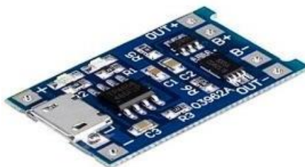
Fig.8 TP4056 Charging Module
