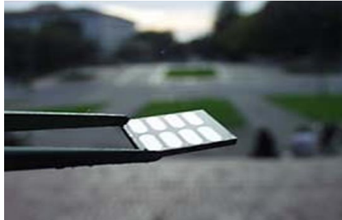
Figure 3- A Panel of eight polymerised solar cell.
