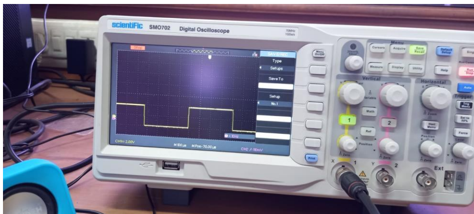
Fig. 4 Output waveform obtained from Audio amplifier
