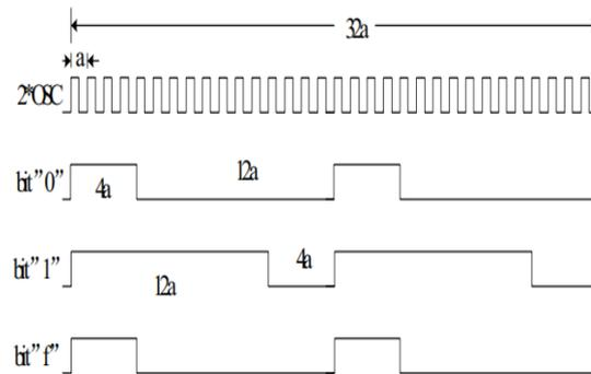
Fig. 4 The trigger timing.
