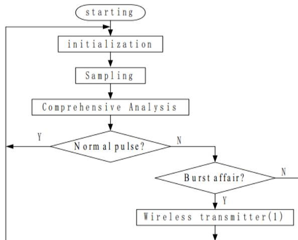
Fig 5 The pulse-monitoring and alarming procedure flow.
