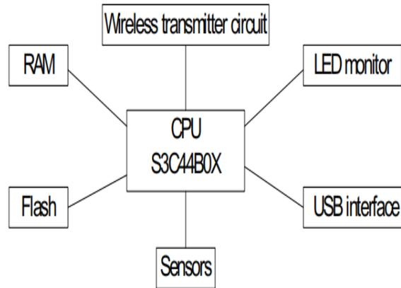
Fig. 2 The whole design structure.
