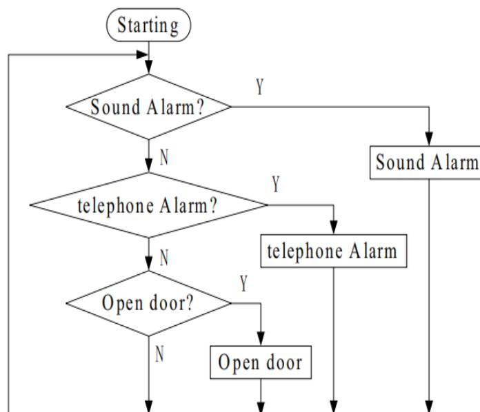
Fig 5 The remote opening door control procedure flow.
