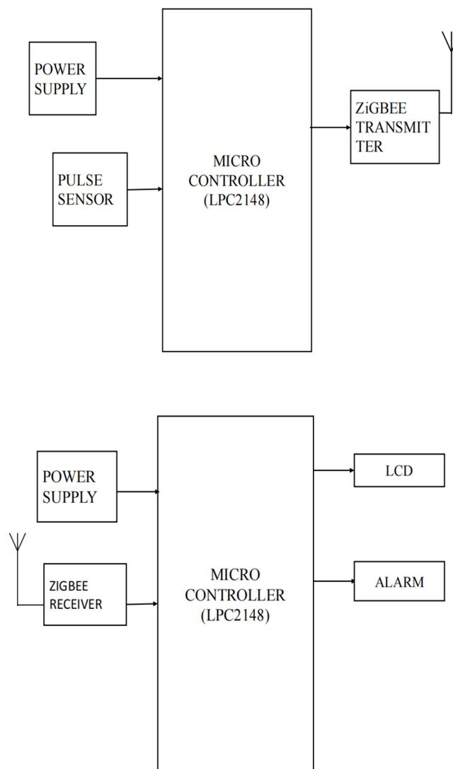
**Fig 1.** Block Diagram.
