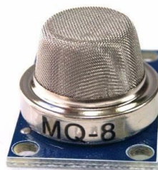
Fig 4 MQ8 Gas sensor
