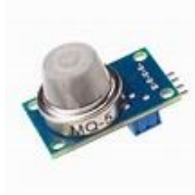
Fig 2 MQ5 EGas sensor
