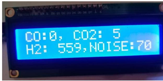
Fig 13 Display of LCD showing the air and noise values
