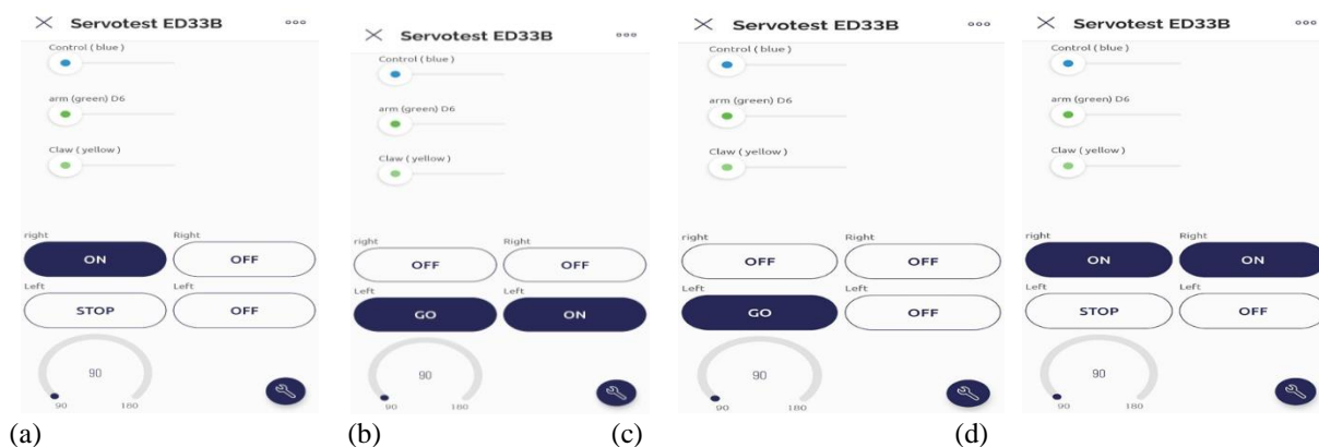
Fig 6.1: (a) To move the Robot towards Right (b) To move the Robot Backward (c) To move the Robot towards Left (d) To move the Robot Forward
