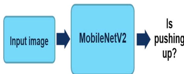
Fig 6: Pushup recognition network based on MobileNetV2
