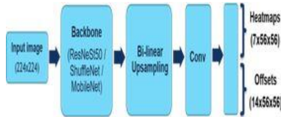
Fig 4: Our proposed architecture - Built from scratch
