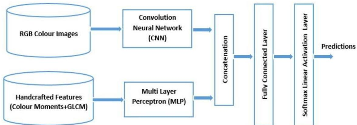
**FIGURE 1. Proposed cascaded ensemble deep learning model has one branch that accepts the extracted features as numerical data and another branch that accepts colour images**
