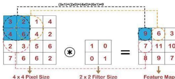
Figure 2. Illustration of the convolution process
