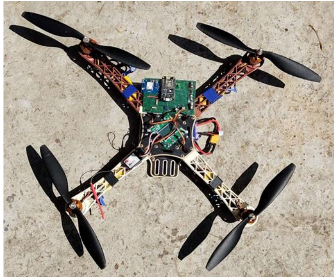
Fig. 7. Drone along with the Geiger Counter
