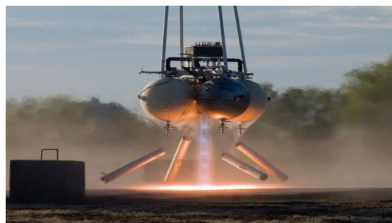
Fig 1. Armadillo Aerospace's quad rocket vehicle showing shock diamonds in the exhaust plume from its propulsion system.
