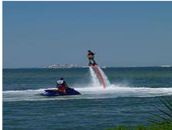
Fig 6. Flyboard with its distinctive configuration of having the nozzles located below the pilot's feet
