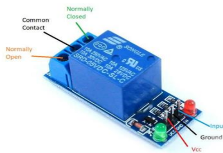
Figure.2 5V Single-Channel Relay Module
