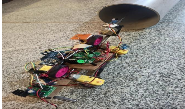
Fig 3.1: Proposed Pipeline Inspection Robot
