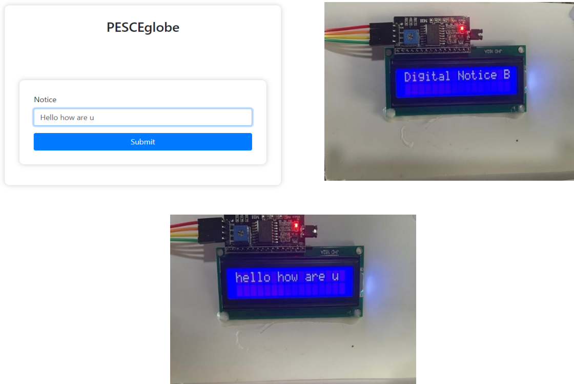
Fig.10: UI interface of digital notice board and the text messages displayed.
