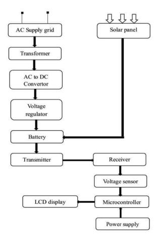
Fig 1: Block diagram of Solar Wireless Electric vehicle charging system
