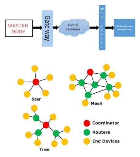
For that using ZigBee is best way which have different network topologies. ZigBee is a low-rate task group 4 personal area network task group. It is a form of home networking technology. A technological standard called ZigBee was developed for managing and sensing the network. Since ZigBee is the Personal Area Network for Task, Group 4 and was developed by the Zigbee Alliance, it is based on IEEE 802.15.4.
