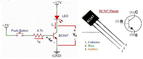
Base-Emitter Junction: When you apply the base current, it causes a forward bias across the base-emitter junction, allowing the transistor to enter its active region and conduct.
