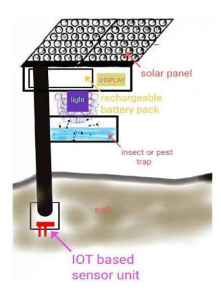
**Pest control unit:** Pest control unit is used to control the pest in agriculture field. In the evening, when the harmful pests cover the crop fields, the solar lamp will switch on automatically and attracts the insects that may destroy the crops. Attracted insects end up in a water-filled basin or trap to a oil paper. Lamp is charged by using solar panel in day hours.
