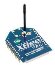
In a Zigbee network, data transmission occurs between three types of devices: the Zigbee coordinator, routers, and end devices (also known as end users). Here's how data transmits between these devices:
