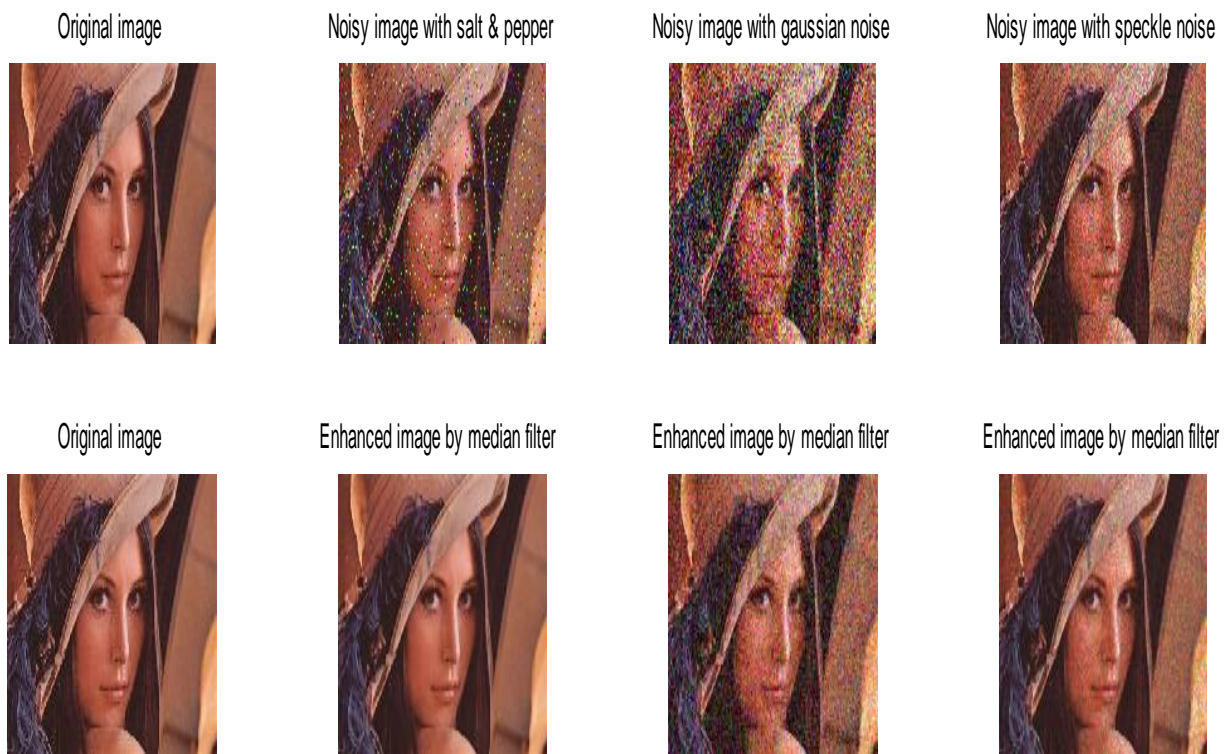
Figure5 :Original Lena image, noisy image with salt and pepper, Gaussian, Speckle noise, and enhanced images using median filter, respectively.
