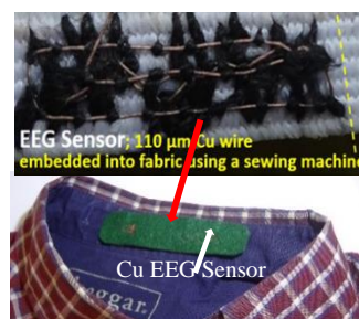
Fig. 8 Technology of EEG sensor embedded in shirt collar that also contains Bluetooth wireless circuits.
