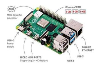
Raspberry Pi serves as the brain of the autonomous vehicle, acting as a central processing unit. It runs the main software stack that processes sensor data, controls the vehicle, and makes decisions. Utilizes its computational power for real-time data analysis, path planning, and decision-making. Communicates with other components and sensors to orchestrate the vehicle's movements.
