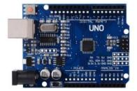
Arduino boards are responsible for interfacing with various sensors and controlling actuators. They manage sensor data, such as GPS, ultrasonic sensors, and IMU, and send it to the Raspberry Pi. Arduino boards can also control servos, motors, and other actuators for vehicle movement. They provide low-level control and real-time responsiveness to ensure safe and precise operation.
