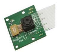
The Raspberry Pi camera is used for capturing visual data, providing a critical input for navigation. It continuously records the surroundings of the vehicle, allowing it to detect and identify objects, lanes, and obstacles. The camera's data is processed by computer vision algorithms to make informed driving decisions. It aids in lane tracking, object detection, and image recognition.
