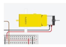
$2^{nd}$  motor = -344 rpm (same as  $1^{st}$  motor but in reverse direction because the motors are placed parallel to each other.
