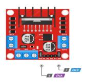
The L298 motor driver is a crucial component for controlling the vehicle's motors. It interprets the commands from the Raspberry Pi and Arduino to regulate the speed and direction of the motors. Ensures the autonomous vehicle can navigate, turn, and stop as per the control algorithms. Offers motor protection and efficiency, preventing overheating or overloading.
