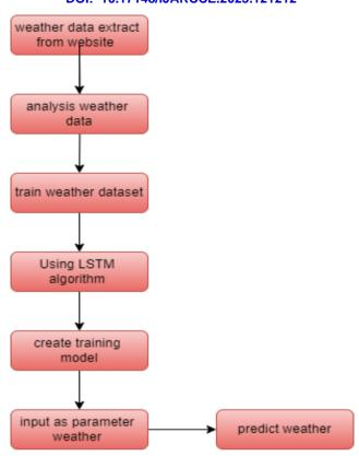
When training an RNN with LSTM units, we follow a supervised approach. We use an optimization technique like gradient descent, coupled with backpropagation through time, to calculate the necessary gradients for adjusting each weight within the LSTM network. This adjustment is done in alignment with how the error at the LSTM network's output layer changes concerning the specific weight.
