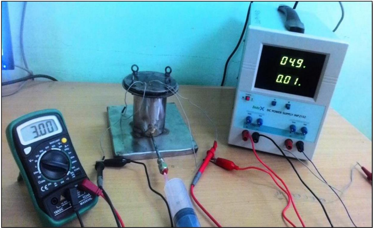
Figure 5. Biogas Leakage Measurement
