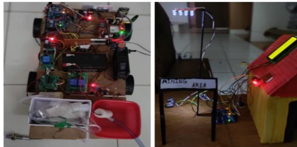
Fig.: 3 Prototype of UDR and Base station model
