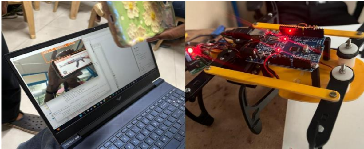
Fig 5: missile detection, if any guns, bombs, knives are detected through laptop camera red LED will be on and immediate buzzer will be on.
