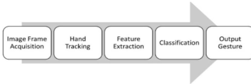
Figure 3: Workflow of hand gesture recognition
