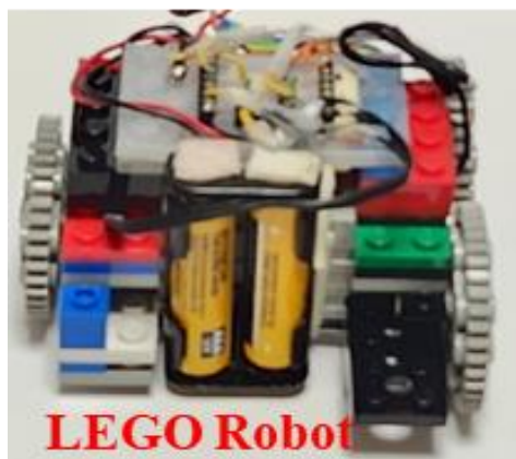
Fig. 5 MUSE-2 controlled LEGO robot in progress.
