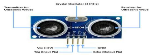
Fig 8: HC-SR04 ULTRASONIC SENSOR
