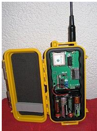
Fig 1.1: APRS beacon transmitter with GPS receiver.
