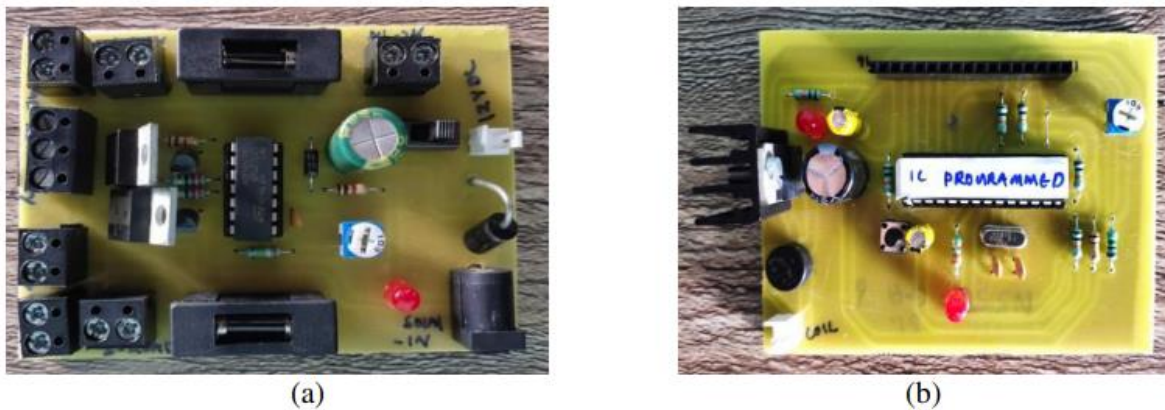
Fig.2. Printed Circuit Board (a) Controller for Solar Charger (b) PCB for Microcontroller
