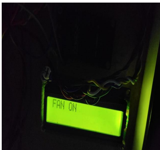
Fig 6 : if a fan image detected through laptop camera fan is On and to turn off again show fan image to camera
