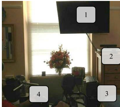
Figure 2: Actual bedroom setup with 1) television, 2) Kinect, 3) computer, and 4) wheelchair with voice activated remote control
