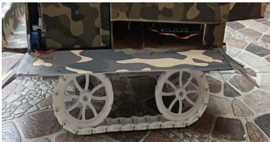
Fig 7: Rover Movement Chain Wheel
