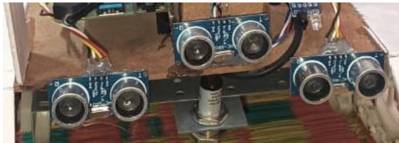
Fig 3: Ultrasonic sensor for Obstacle Detection
