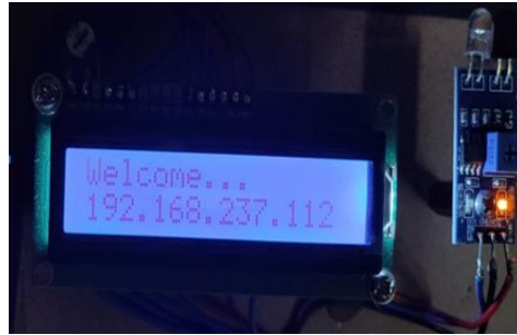
Figure 4: Lcd showing the IP address for payment page
