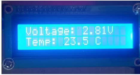
Figure 3: Lcd showing the Voltage level and temperature
