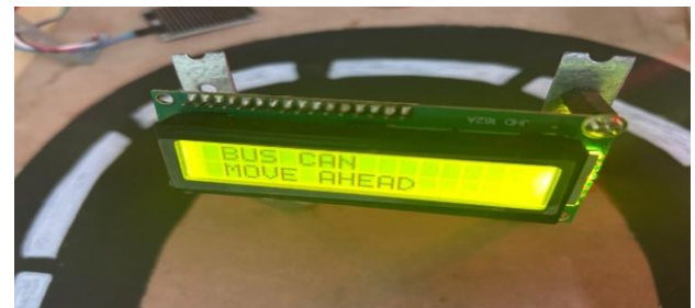
Fig. 12. Images are detected in laptop camera and then in hub model LCD will display that PRIORITY FOR BUS GIVEN and again it will display BUS CAN MOVE AHEAD
