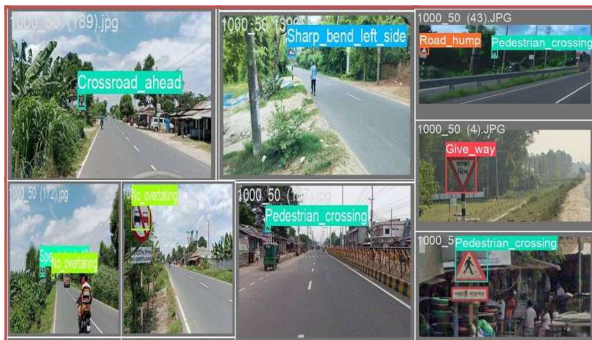
Fig. 5. Our test dataset's sample detection outcomes across a range of test settings.
