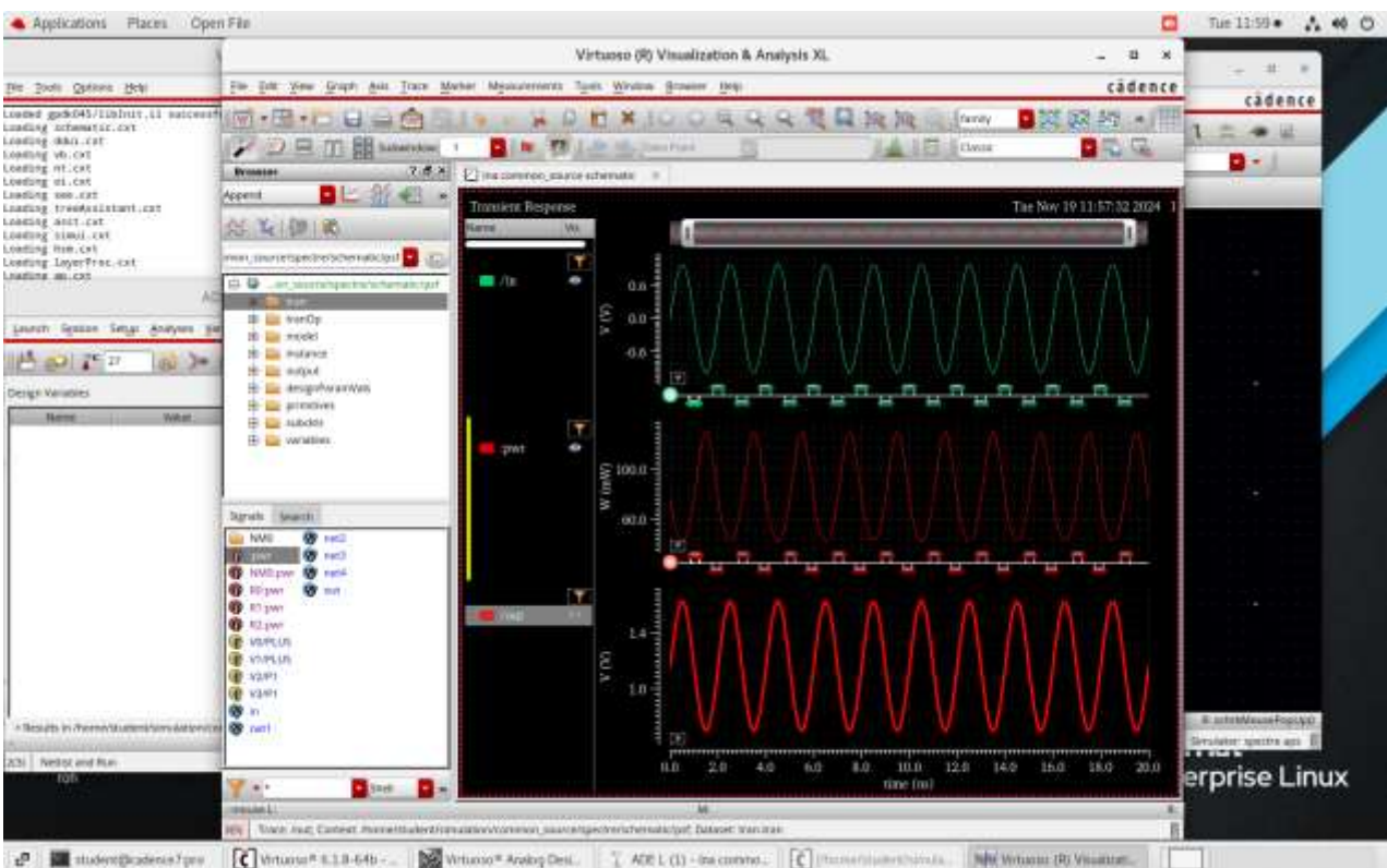
Figure 4- Transient analysis after parasitic extraction.
