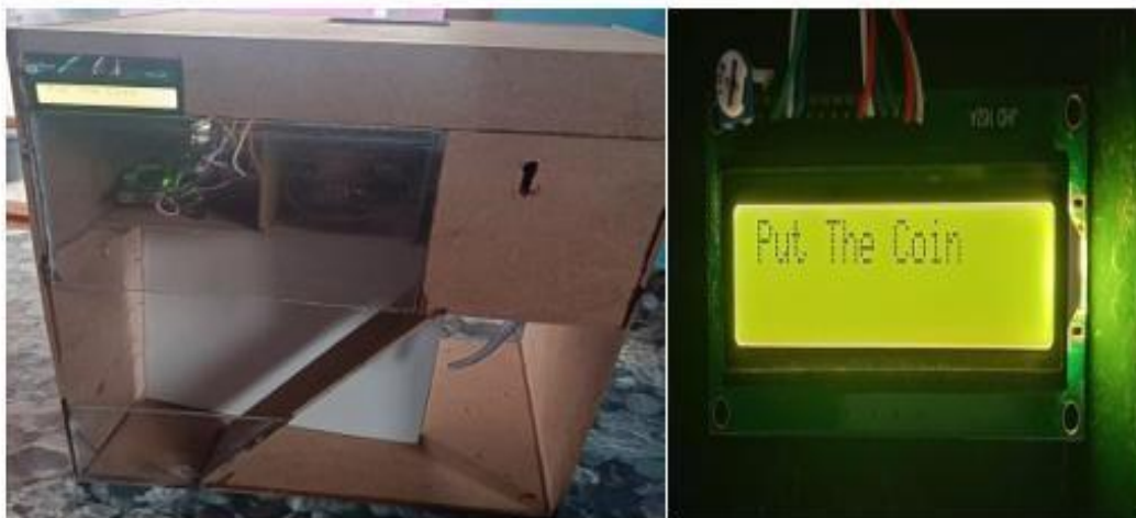
Fig.: 4 WATER ATM Display the Coin Detection
