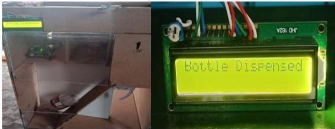
Fig.: 5 WATER ATM Displaying Bottle Dispensed
