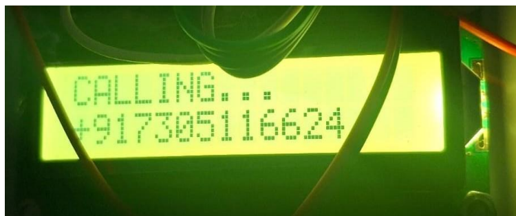
Fig 7.3 LCD Display displaying Alert Notification (Calling)
