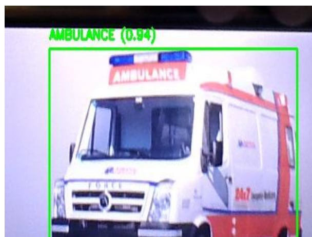
Fig 6: Ambulance or any emergency vehicle being detected by YOLOV8 tool at 0.94 accuracy.
