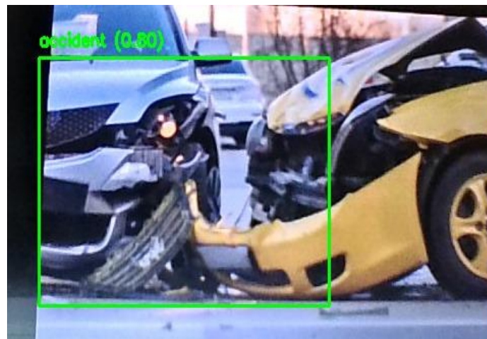
Fig 7: Accident being detected by YOLOV8 tool at 0.80 accuracy.
