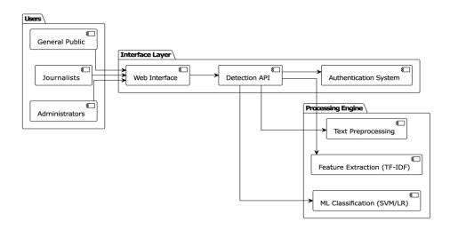
This diagram shows the structure of the fake news detection system. Users like general public and journalists connect to a web interface. That interface links to a detection API with security. The API then goes to processing parts: text cleaning, feature making with TF-IDF, and ML models for classifying news as verifiable or forged. It is simple way to see how the system works from start to end.
