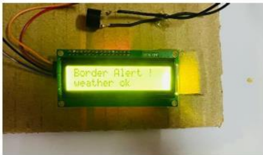
Figure 6 a) and b) illustrates the message generated under unsafe condition on LCD and COM Port
