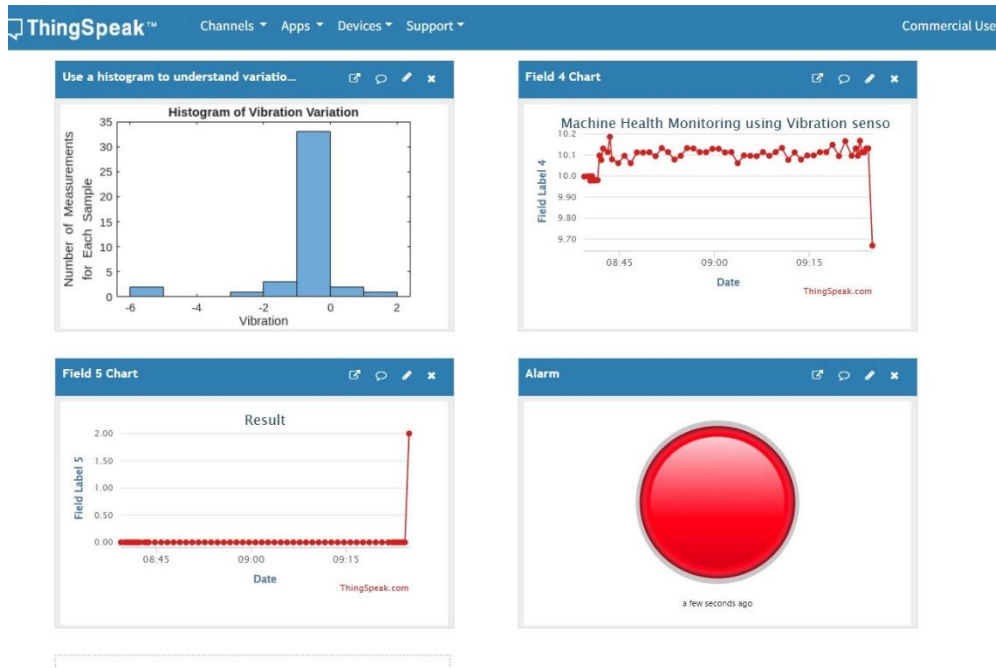
Fig. 5 Thingspeak visualization with alarm
