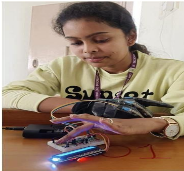
Fig 4: System Testing of Myoelectric Gesture Recognition Glove for Stroke Rehabilitation
