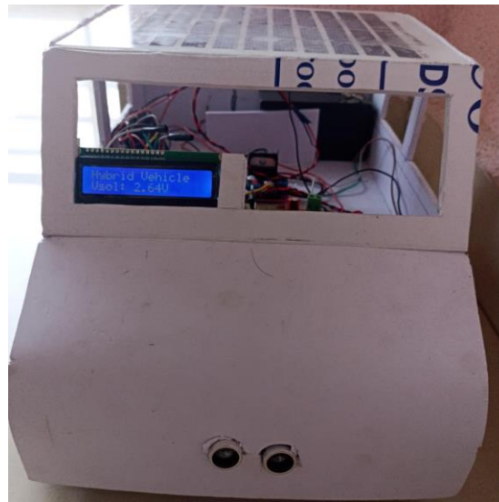
Fig. 4.4 Battery charging due to solar energy.
