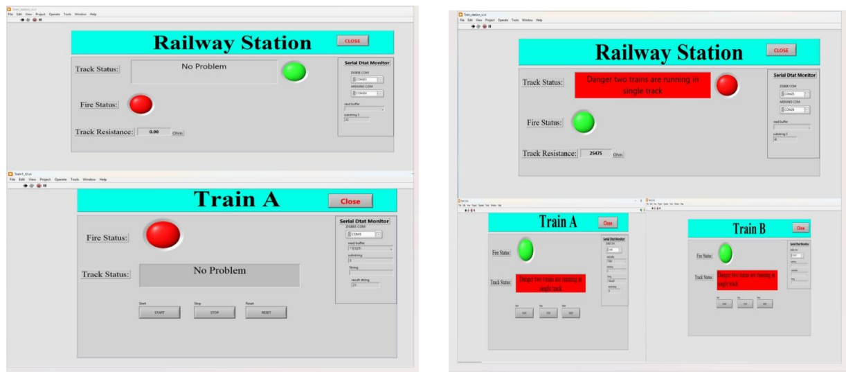
Fig.8: LabVIEW interface presenting combined fire detection and collision avoidance system
